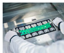
A battery module is prepared for connection by laser welding.
